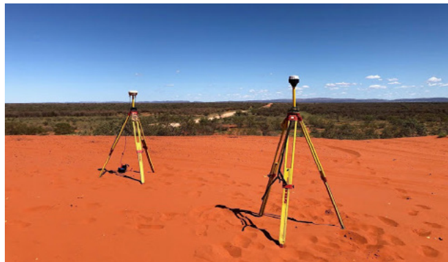
Figure 2 Emlid Reach RS2 and Trimble R63 base units established for radio corrections range test. (Chris Nichols, BBS)
