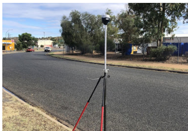
Figure 13 Emlid Reach RS2 setup on a CRM for AUSCORS-based RTK testing
