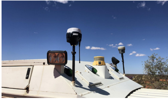
Figure 3 Emlid Reach RS2 and Trimble R10 rover units mounted on survey vehicle for radio range test (Chris Nichols, BBS)
