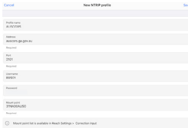
Figure 12 Screenshot showing the NTRIP profile used for the performance test with corrections from AUSCORS
